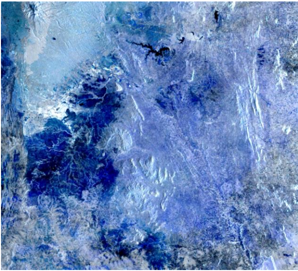
Figure 22: Example of multi-temporal min-mean-max of all VH images acquired during the long wet season March-August 2019 over the Nairobi area
