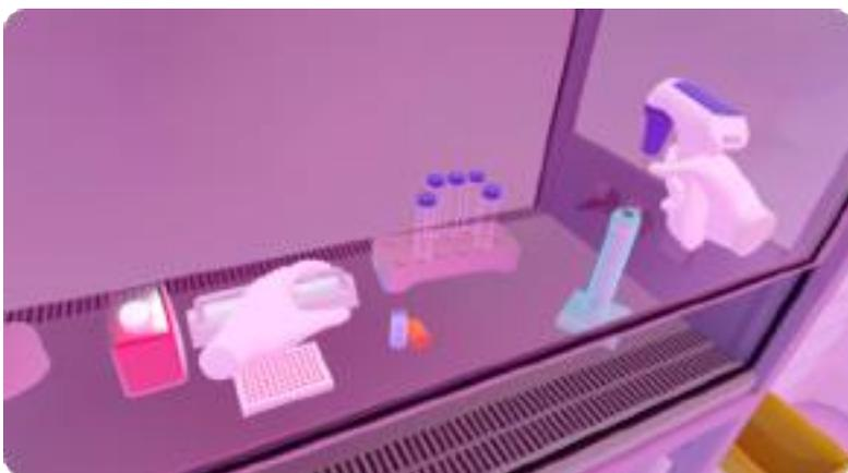
Now we have to exchange the pipette, to make sure it is sterile for its use with neurons. Hold the pipettor into the pipette dispenser to your right.
