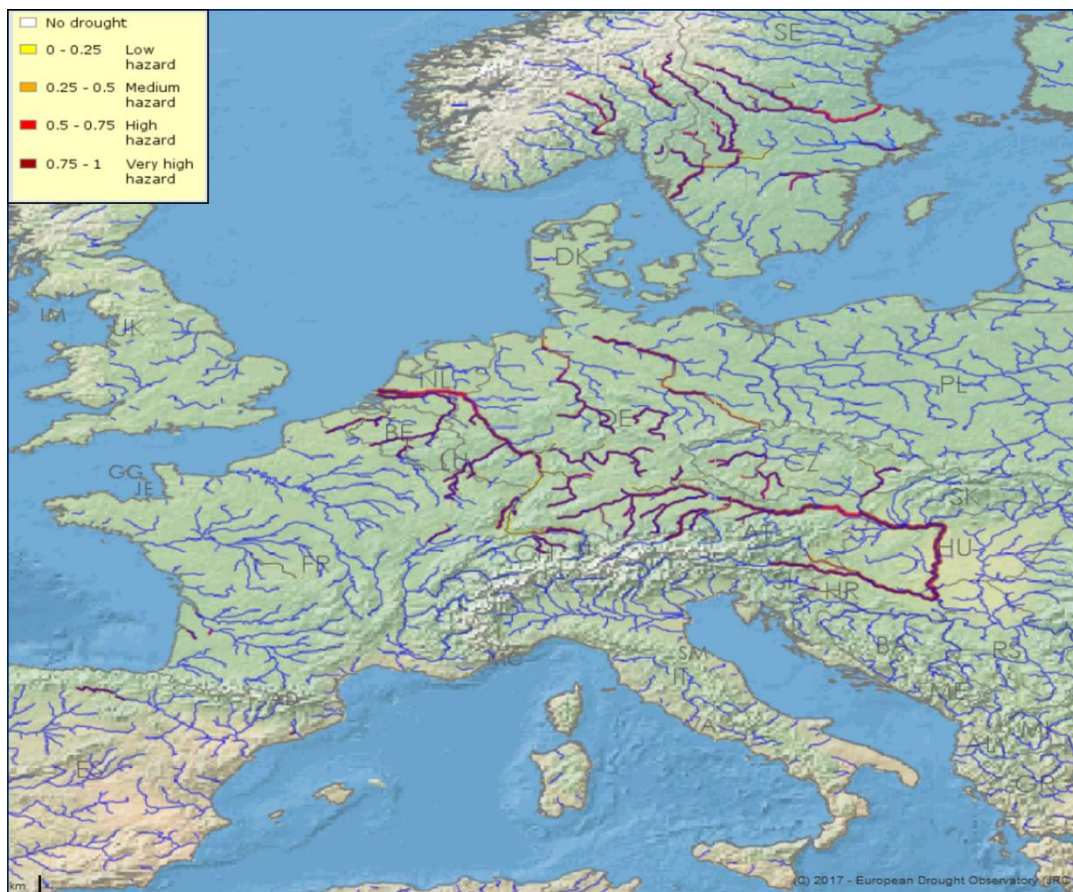
Figure 1: Example of the continuously updated LFI indicator, implemented within the Copernicus European Drought Observatory (EDO), showing the hydrological (or streamflow) drought status computed for the 10-day period 21-30 June 2017.
